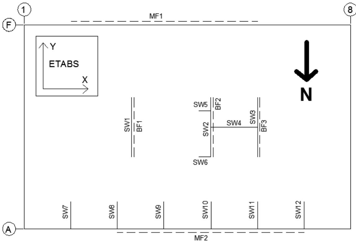
Figure 18: Labeling of Lateral System Elements (Source: Chavanic)
