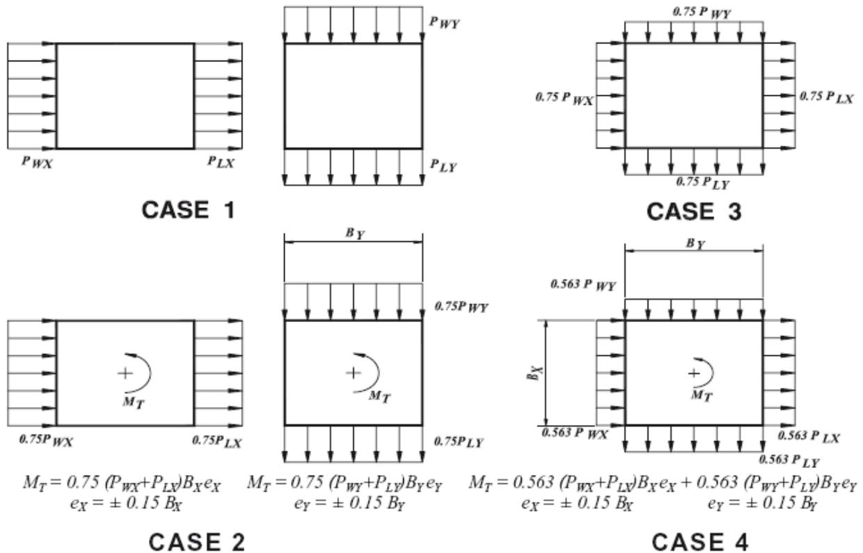
Figure 23: Design Wind Load Cases (Source: ASCE 7-10 Figure 27.4-8)
